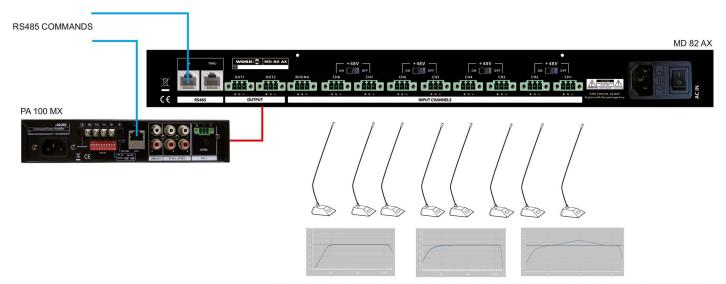
HIGH-PASS/LOW-PASS FILTERS & GAIN LEVEL ON EACH CHANNEL CAN BE CONFIGURED USING THE FRONTAL ENCODER OR RS485 COMMANDS FOR EXTERNAL DEVICE
